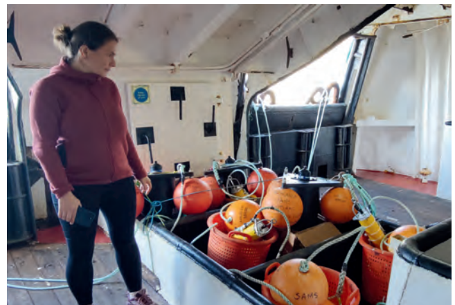
Minke whale monitoring set-up and PAM devices
