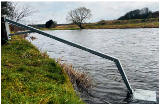
Flood-resistant structure for sonar device
